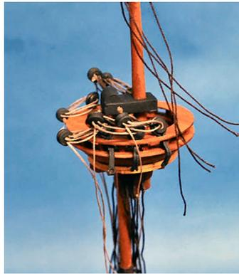
The first image shows the floor of the fighting top and the basket sides, which Allen turned on a lathe.
