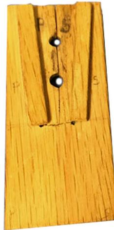
Here is the jig that Allen built to rig his deadeyes. The frame locks the deadeyes into the correct spacing and the holes in the back of the jig allow for passing line through the deadeye holes.
